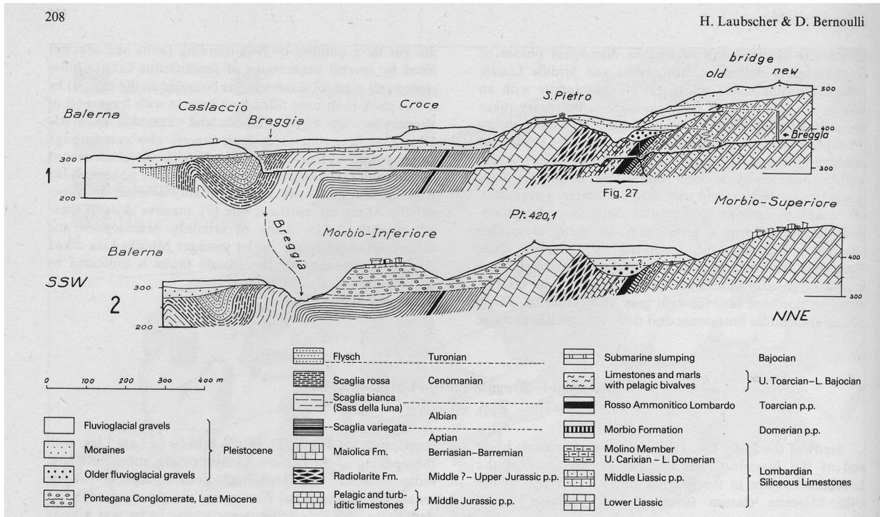
Fig 26 Geologic profile through the Mesozoic sequence of the Breggia valley (after L. Vonderschmitt 1940, modified).
