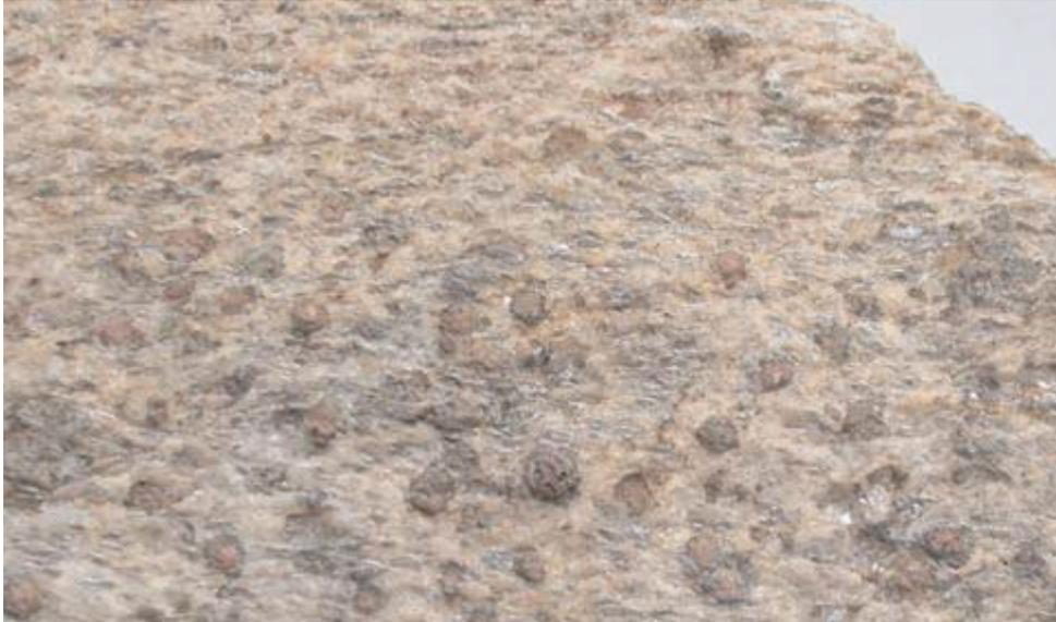
Fig. 29 - Typical character of the quartz-rich metasediments. The main variation that can occur is in the inclusion, character and abundance of garnet. Note in this sample that the intensity of shear increases towards the top and that the abundance of garnet decreases with the increase in intensity of shearing. FOV ~9 cm.
