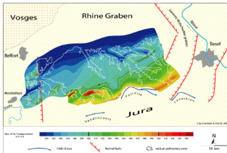
**Fig. 6:** Contour map of the base of the Pliocene (3.2-2.6 Ma) Sundgau gravel deposits W of Basel. Assuming an originally planar base of these braided river deposits, the contours indicate folding with an amplitude of up to 200m. This indicates substantial tectonic movements during the last 3 Ma, post-dating thin-skinned Jura-tectonics. From Giamboni and Schmid, work in progress. (Large image)
